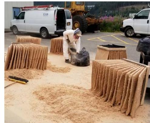
But someone's got to do it. Ever wonder where all of that saw dust goes at our TEC wood shop? We have a saw dust collection system that has vacuum hoses connected to all of the equipment including a few floor collectors. Much of the sawdust gets collected in 55 gallon drums that we regularly empty. The rest clings to the vacuum filter bags where we have to brush it off a couple times a year. It's such a dusty job that we wear protective clothing and respirators.
